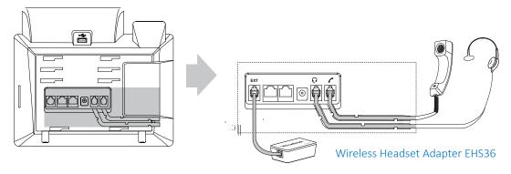
Note: The headset or wireless headset are not included and needs to be purchase seperatelt if interested. The EXT port can also be used to connect the expansion module EXP40. For more information on how to use the EHS36 and EXP40, refer to Yealink EHS36 User Guide and Yealink EXP40 User Guide.
