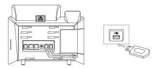
Note: The USB port can also be used to connect Bluetooth USB dongle BT40 or Wi-Fi USB dongle WF40. The Bluetooth USB dongle BT40 or Wi-Fi USB dongle WF40 should be purchased separately. For more information on how to use the BT40 and WF40, refer to Yealink Bluetooth USB Dongle BT40 User Guide and Yealink Wi-Fi USB Dongle WF40 User Guide.
